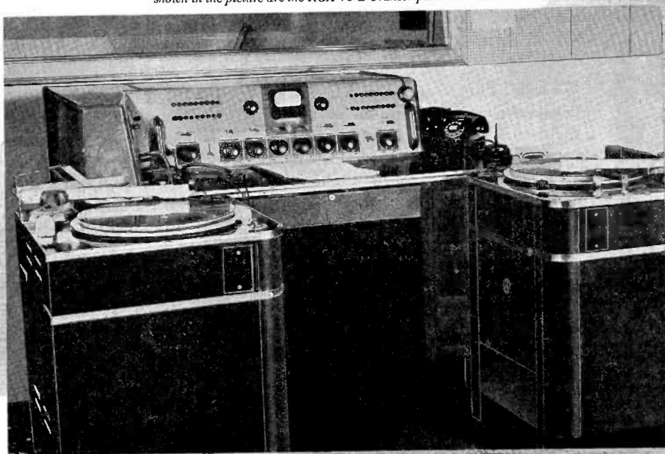
The RCA 76-B Console in the control room of WLOU. Also shown in the picture are the RCA 70-B Transcription Turntables.
